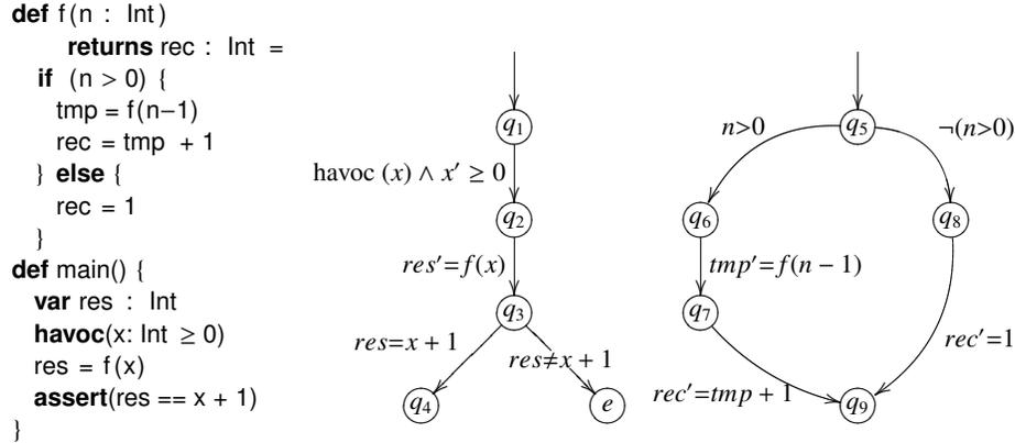
**Fig. 1.** A recursive program and its control flow graph (see Sect. 3).
